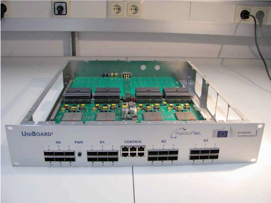
Figure 8: UniBoard2 + backplane test board in enclosure
