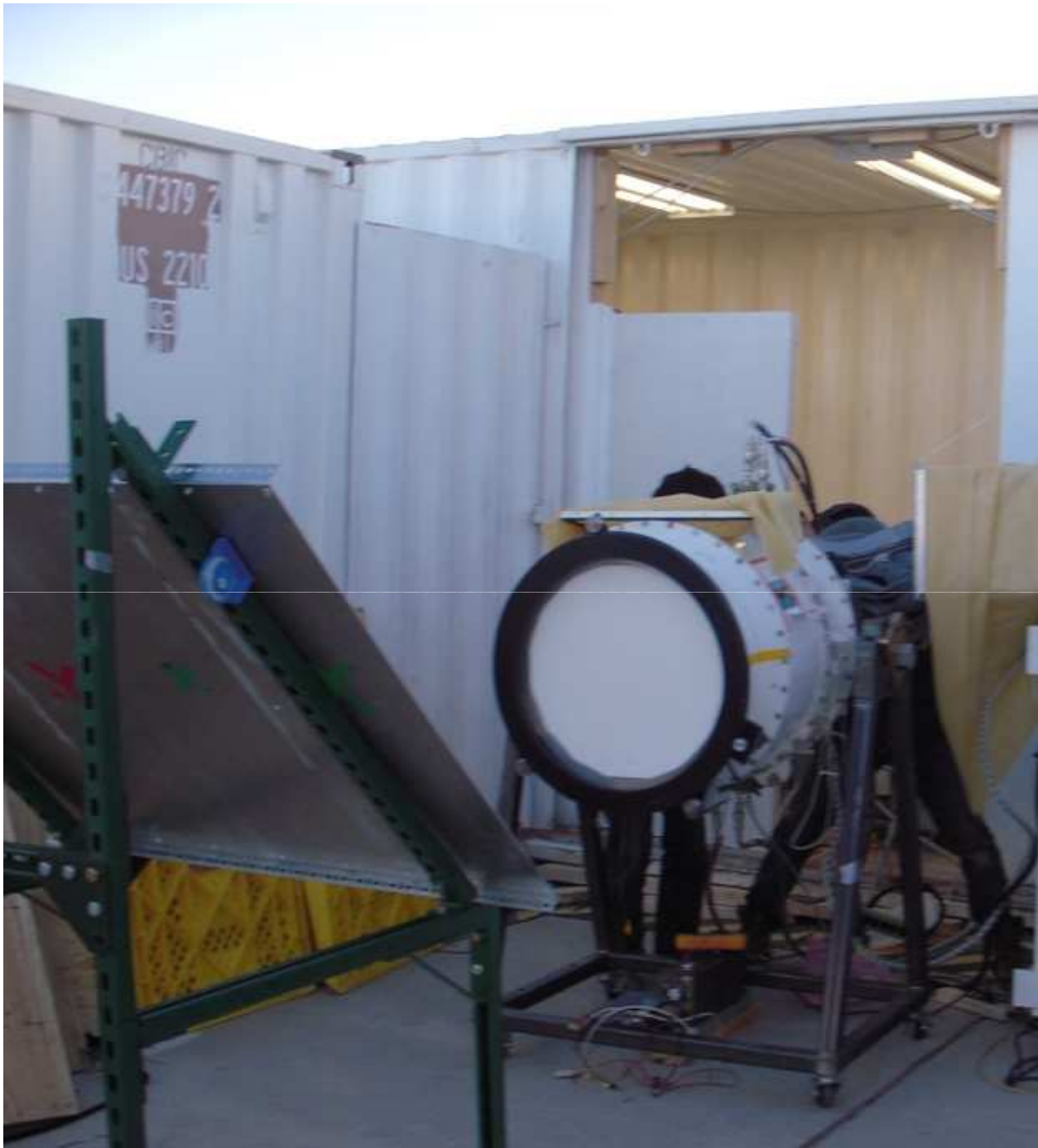
Rotating wiregrid at the site looking at the sky (via metal plate)
