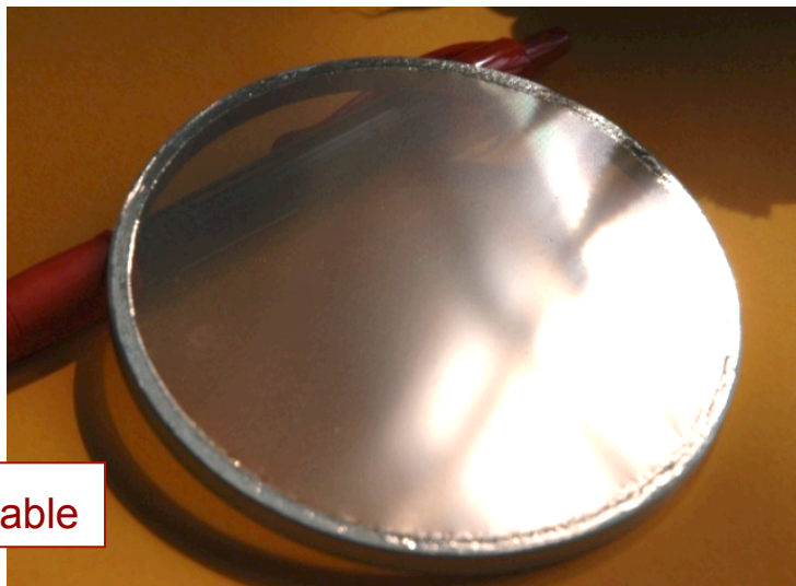
Single Metal Mesh on dielectric substrate
