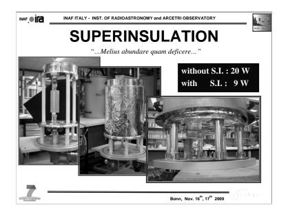
All the cooled metal parts are covered by a blanket acting as Superinsulation.
