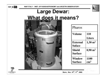
The picture shows the Pharos vacuum chamber with his typical dome. The DC connectors and RF output are located on the back of the cylinder.
