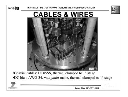
All the 21 coaxial cables are the UT85SS. The coax cables are all thermal clamped to the 1° stage cryocooler.
