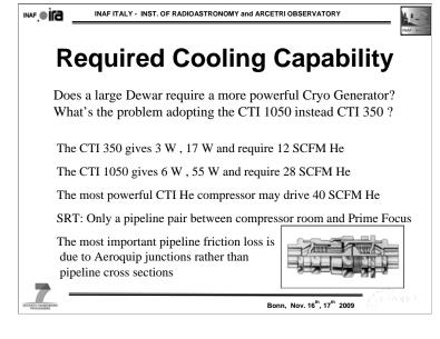
An extensive study has been commissioned to a  $3^{rd}$  part has shown that, for a 100 mt long pipeline, the most important contribution to the He flow friction loss, is due to the Aeroquip junctions rather than the ling pipelines.
