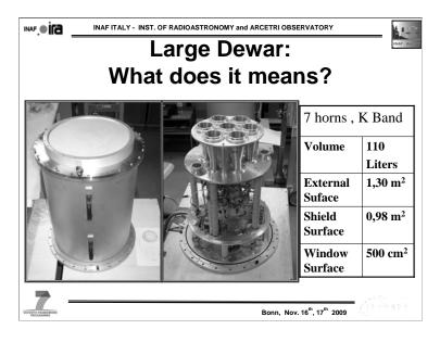
The pictures shows the Faraday 18-26.5 GHz, Dewar array, on the left the whole vacuum chamber, on the right the core of the array. The seven horns are cooled down to the  $2^{\circ}$  stage (i.e. 20 K).
