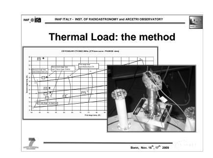
Many are the possible methods to measure the thermal load. The adopted method take advantage by experimental activity. The measured data has been superimposed over the graphics coming from the factory. A necessary initial calibration has been done in order to remove the offset.
