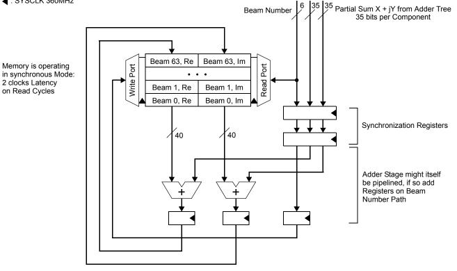
Figure 11: Accumulator Stage (Basic Form)
