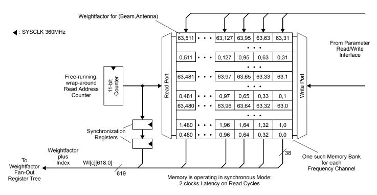
Figure 13: One Weightfactor Memory Bank
