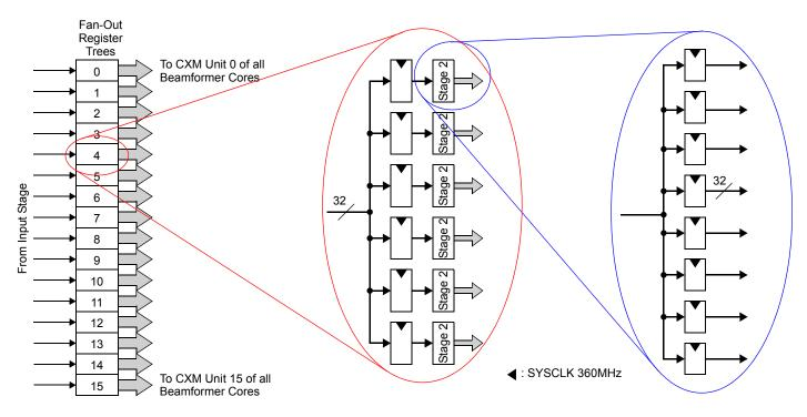
Figure 5: Input Fan-Out Register Tree
