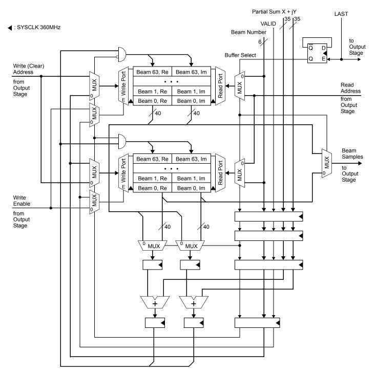
Figure 12: Double-Buffered Accumulator Stage
