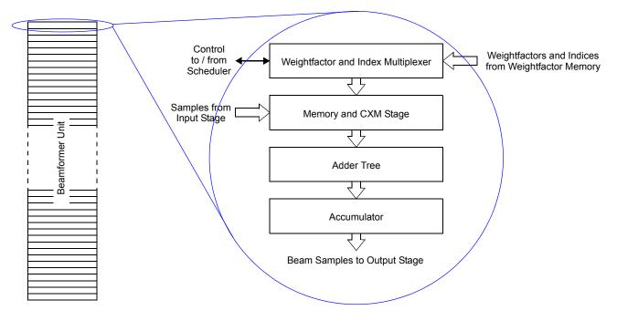
Figure 6: Beamformer Core Block Diagram
