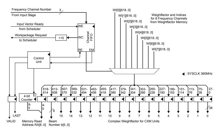
Figure 7: Weightfactor and Index Multiplexer
