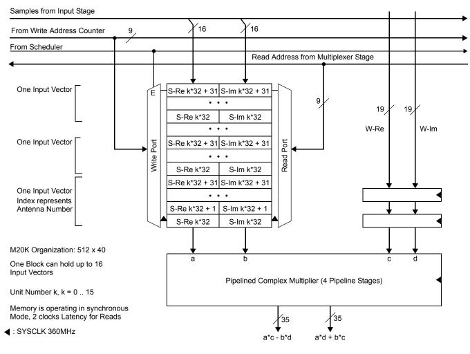
Figure 8: One Sample Memory and associated CXM Unit
