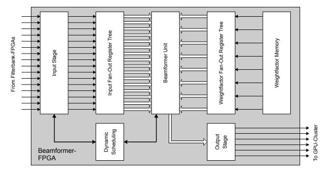
Figure 3: Beamformer-FPGA Block Diagram
