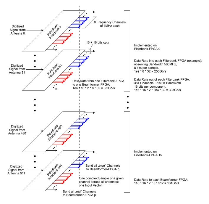
Figure 1: General Filterbank Architecture
