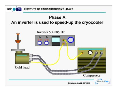
The way to speed up the cool down time is to speed up the cold head. What does happen if we drive the cold head with an higher frequency?
