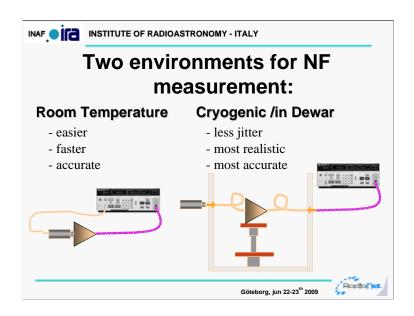
Two are the convenient environments where perform the Noise Figure (or Noise Temperature) measurement.
