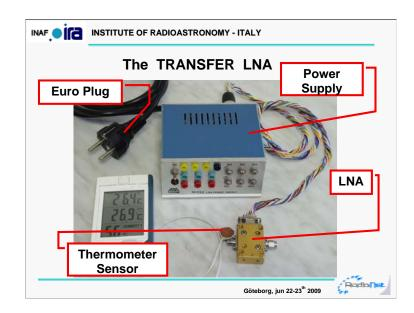
The transfer LNA will be shipped into a cardboard box. It's as plug'n play as possible. Not shown here , the ferrite circulator.
