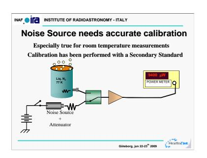
This is a sketch of the Noise Source calibration procedure.
