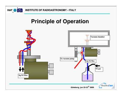
A thin stainless steel pipe is wrapped around the two stages.
