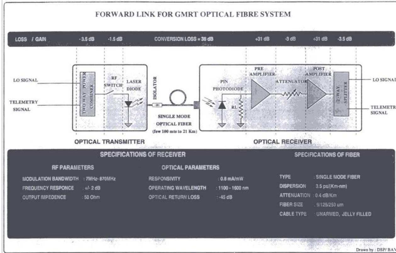
Forward link transmits a pair of LO Reference Signals at 105 and 200 MHz as well as Telemetry FSK signal around 18 MHz
